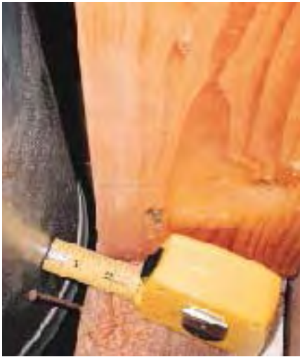
Figure 21. As a matter of life safety, combustion appliance vent pipes must have proper clearance to combustibles. The guidelines are usually stamped right on the appliance itself.
